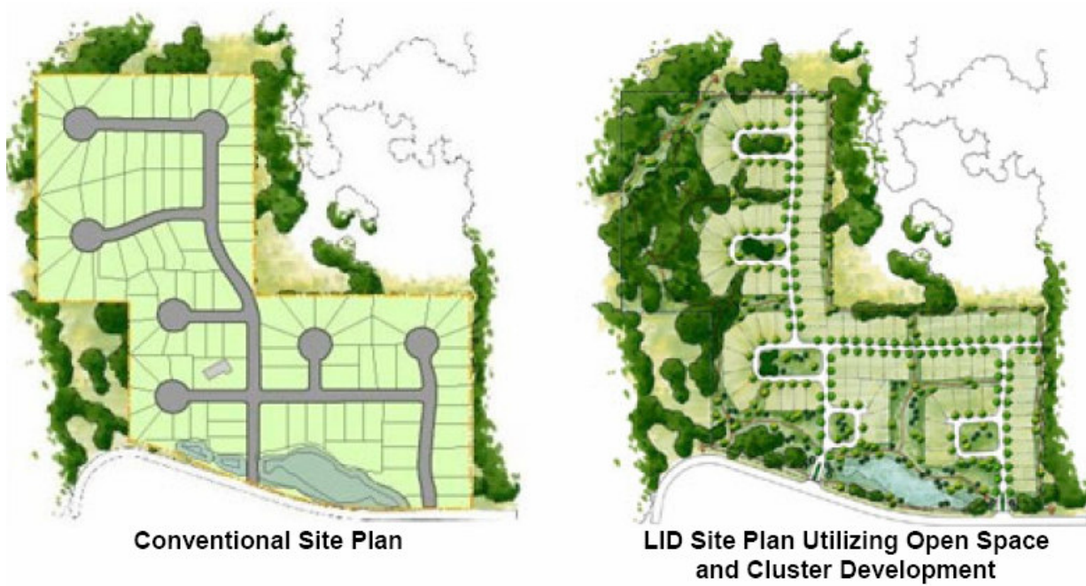
Figure 1. Comparison of Conventional Site Plan and LID Site Plan on the Same Site
